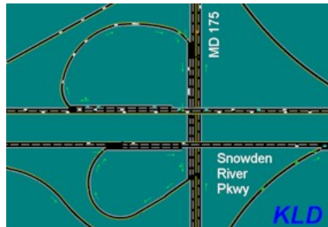
Figure 2.11: WATSim simulation of proposed design for a freeway/arterial interchange in Howard County, Maryland performed by KLD Associates, Inc.
